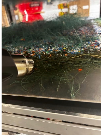
Figure 20: The melted edges of the “rough sheet” were achieved using a heat gun. ROTR had hoped that a heat gun might help the press reach Nylon melting temperatures, but this was not the case.
