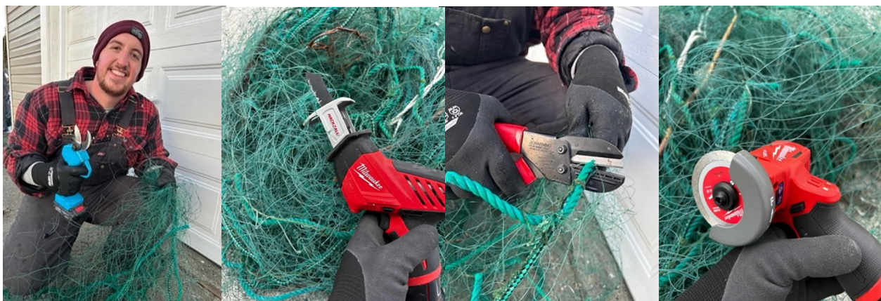
Figure 4: Utilizing a variety of cutting tools to separate and untangle rope from the gillnet. The M12 tool (far right) was the most efficient.
