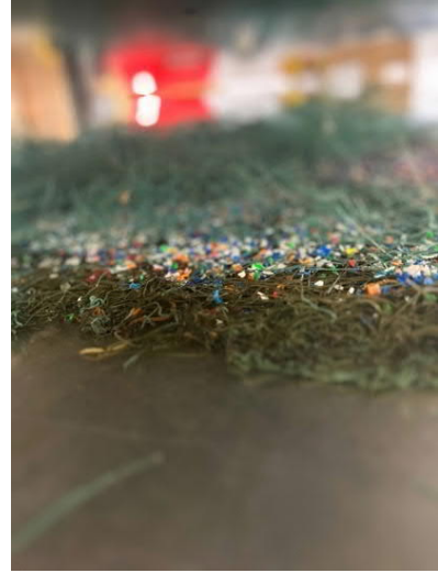
Figure 21: A mixture of compressed gillnet, plastic bottle cap flakes and unpressed gillnet about to be tested in the sheetpress.
