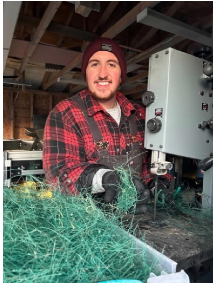
Figure 12 & 13: ROTR purchased a King Canada bandsaw and swapped the traditional blade with a unique “single edge” knife blade. This setup mimics “bandknife” machines used in foam & garment cutting factories. The single edge knife blade was used to prevent “snagging” and improve efficiency.
