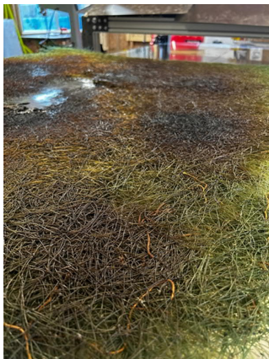
Figure 18: The result from the first test. The machine was heated as much as possible & was left running for several hours but failed to reach the melting temperature of Nylon. The result was a compressed mass of gillnet. Some areas of the net were burnt (likely from debris or dirt) but no melting was visible.
