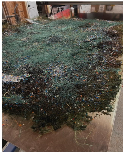
Figure 19: The dark base of the rough “sheet” is compressed gillnet from earlier testing. After making some more adjustments to the press, ROTR wanted to see if the addition of plastic cap flakes & more gillnet would make a difference upon re-pressing. After re-heating and pressing, some of the plastic cap flakes had melted but it was clear that it did help the melting or binding of the gillnet. The sheet was only left in the press for around 15 minutes. A longer melting window will be needed.
