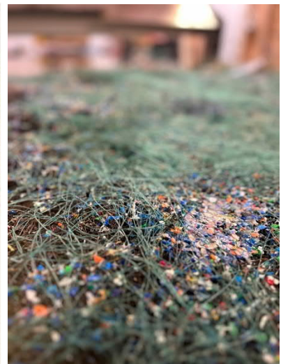
Figure 19: The dark base of the rough “sheet” is compressed gillnet from earlier testing. After making some more adjustments to the press, ROTR wanted to see if the addition of plastic cap flakes & more gillnet would make a difference upon re-pressing. After re-heating and pressing, some of the plastic cap flakes had melted but it was clear that it did help the melting or binding of the gillnet. The sheet was only left in the press for around 15 minutes. A longer melting window will be needed.
