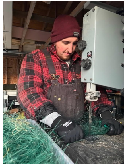
Figure 12 & 13: ROTR purchased a King Canada bandsaw and swapped the traditional blade with a unique “single edge” knife blade. This setup mimics “bandknife” machines used in foam & garment cutting factories. The single edge knife blade was used to prevent “snagging” and improve efficiency.
