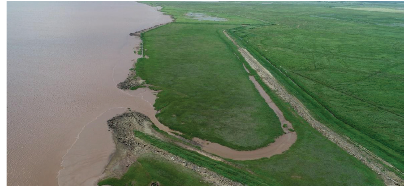
Figure 11. The western Aulac restoration cell 11 years after the seaward dike (left side of photo) was intentionally breached (at what is now the mouth of the creek running through the site; photo taken in July 2022). The restored marsh cell (~11 ha) is bordered by the remnants of the dike on the seaward edge and the new, inland dike (right side of the photo) that runs parallel to it. As of the time of this photo, the marsh surface is blanketed by Spartina alterniflora .
