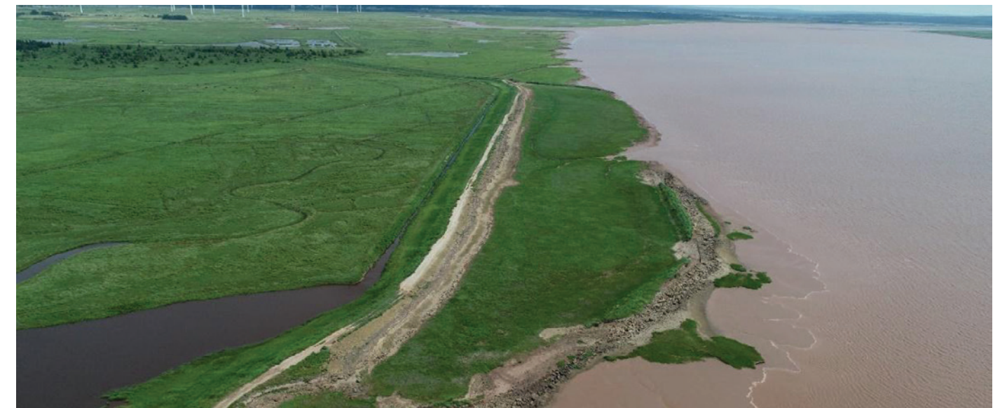
Figure 12. The eastern Aulac restoration cell 11 years after the seaward dike (right side of photo) was intentionally breached (both near the middle of the site and on the far end; photo taken July 2022). The restored marsh cell (~5.5 ha) is bordered by the remnants of the dike on the seaward edge and the new, inland dike (left side of the photo) that runs parallel to it. As of the time of this photo, the marsh surface is blanketed by Spartina alterniflora .
