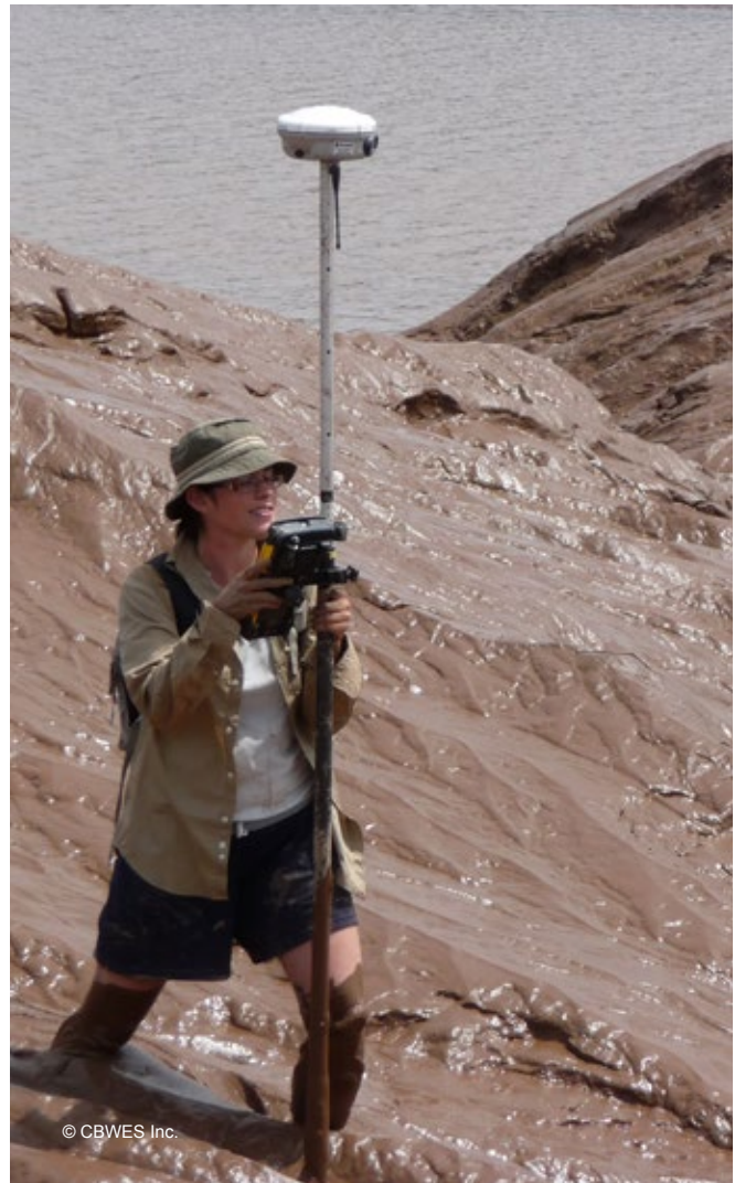
Photo: Jennie Graham from CBWES conducting an elevation survey within a tidal salt marsh channel, Bay of Fundy. The data from research and monitoring activities like this helps CBWES understand the form and function of these dynamic coastal systems and improves the ability to design habitat restoration and climate change adaptation projects.
