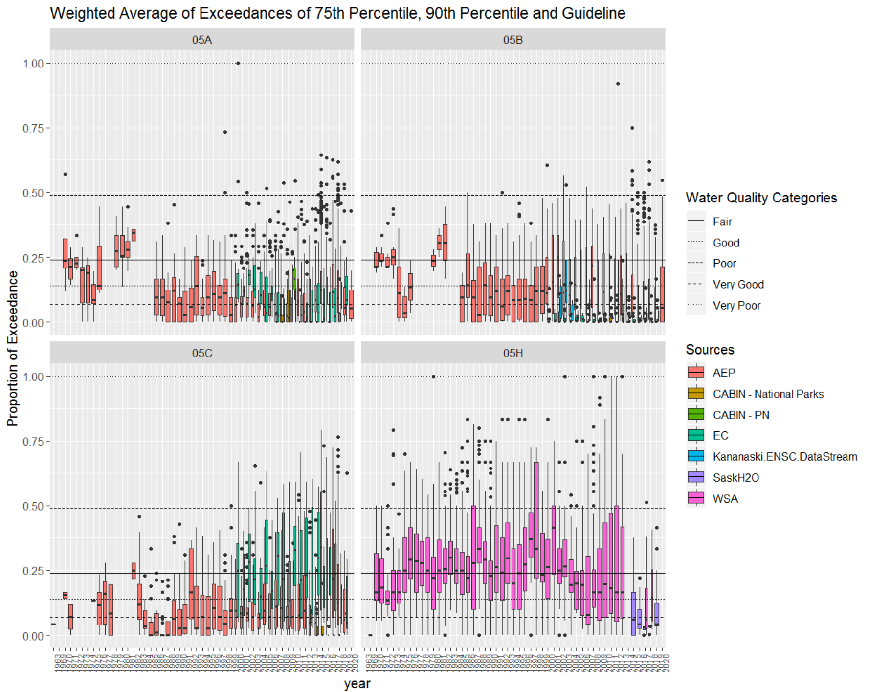
FIGURE. ANALYSIS OF VARIANCE IN EXCEEDANCE OF WATER QUALITY THRESHOLDS OVER TIME FOR MONITORING STATIONS IN THE ALBERTA PORTION OF THE SOUTH SASKATCHEWAN RIVER BASIN, BY CONTAMINANT.
